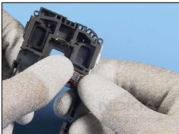
5. Now position the connector side.
