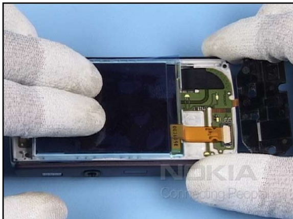
7. Place the display into its compartment.
