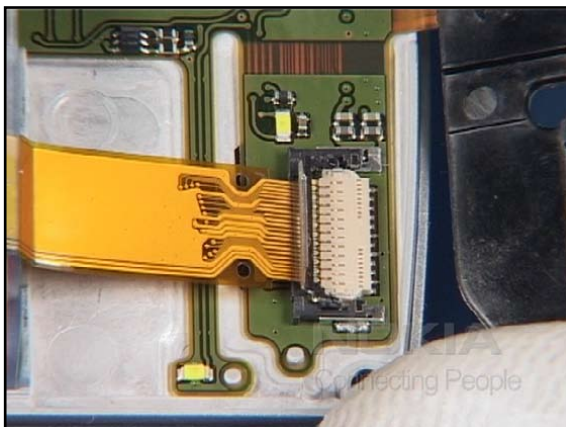
4. Insert the flex foil of the display into the connector evenly.
