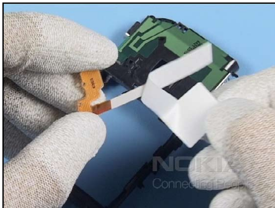
2. Remove the protective film from the 1UJ FLASH MODULE.
