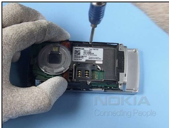
32. Tighten these screws slightly.
