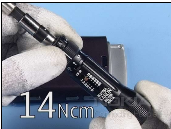
16. Set the correct torque.
