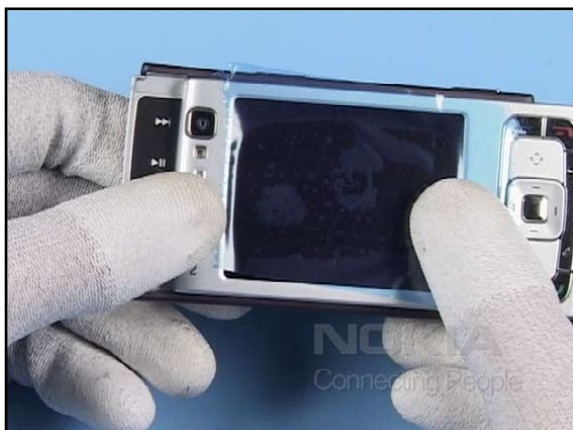
21. Check the functionality of the slider.
