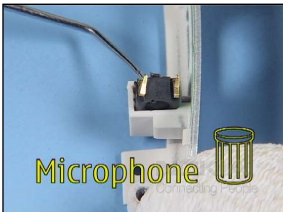
23. Ease out the MICROPHONE and discard it, use a new one when reassembling.
