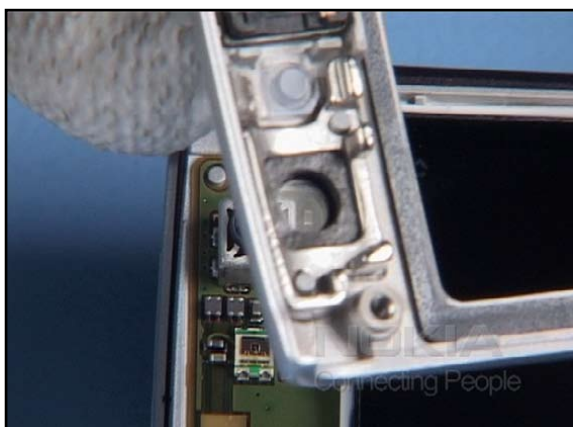
11. Check that the window and camera are clean, otherwise clean it up before going on.
