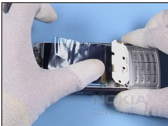
15. Cover the display with a protective film.
