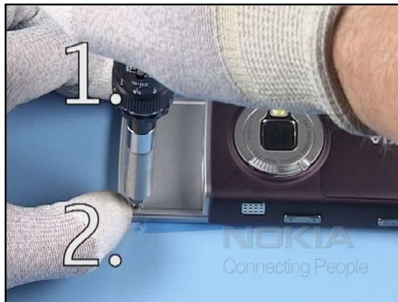
20. Tighten them to the correct torque in the order shown.
