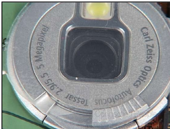
38. Ensure that the protection film is still fitted, otherwise protect it with a plastic film.
