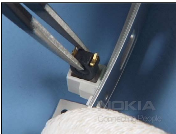
16. Insert the MICROPHONE.
