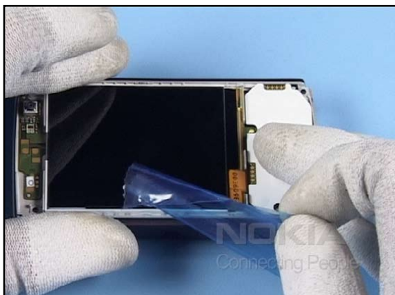
9. Peel up the protection film.
