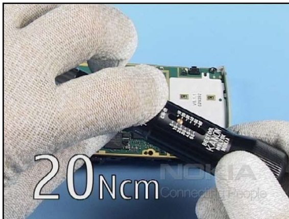
26. Set the correct torque.
