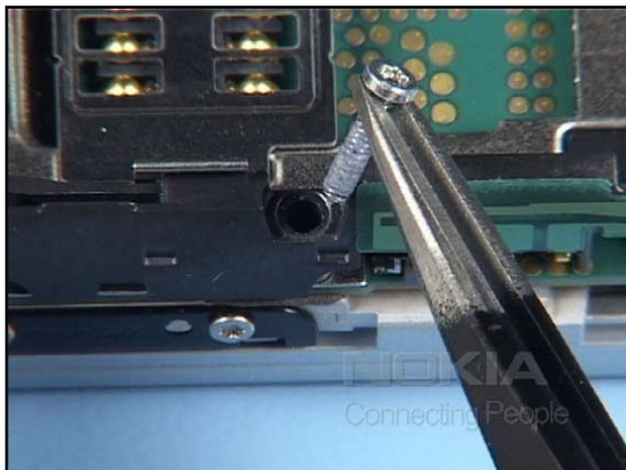
31. Insert the 2 new screws.
