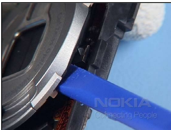
30. Gently release the adhesive of the CAMERA PROTECTIVE SHUTTER MODULE. Mind the hidden switch underneath!
