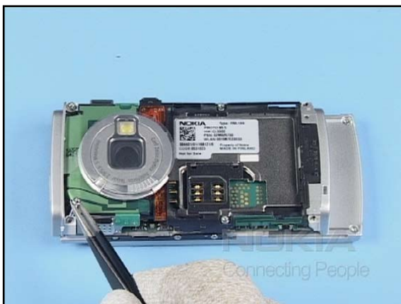
34. Insert the next 2 new screws.
