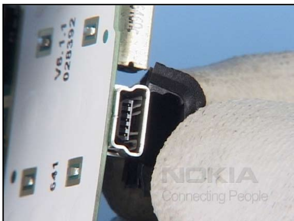
21. Remove the USB SEAL.
