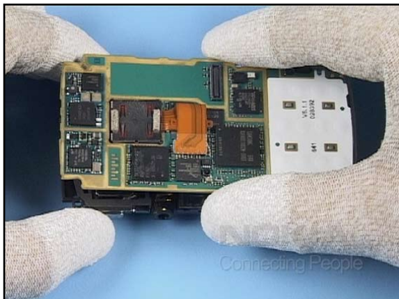
19. Lift up the LIGHT SWAP PWB together with the MAIN CAMERA.
