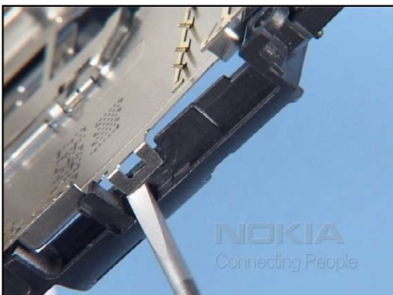
29. and then the second one. Do not touch or bend the gasket. Keep it together with the PWB.
