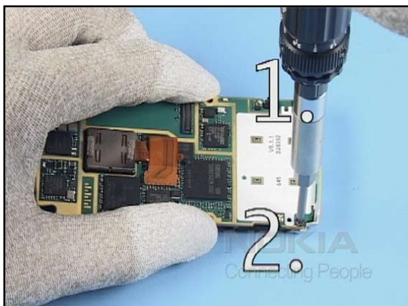
27. Apply the torque in the order shown.
