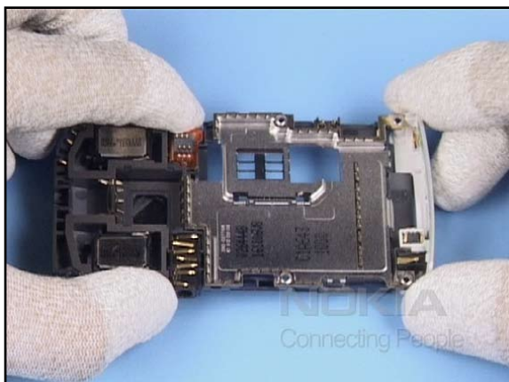
17. Fit the BOTTOM COVER to the CHASSIS now.
