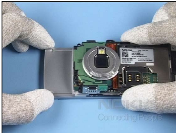
14. Shift out the assembly in order to gain the maximum flex foil length.
