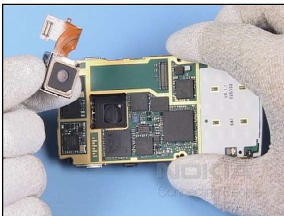
22. Check the camera and the window for cleanness before going on.
