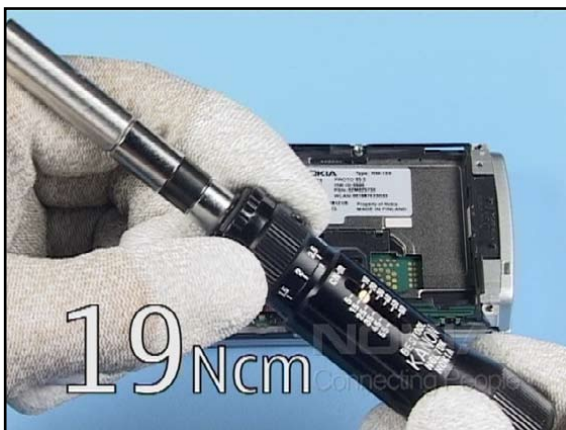
36. Set the correct torque.
