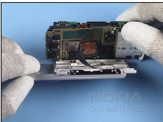
15. Separate the assemblies, keep in mind that the flex foil is still connected.
