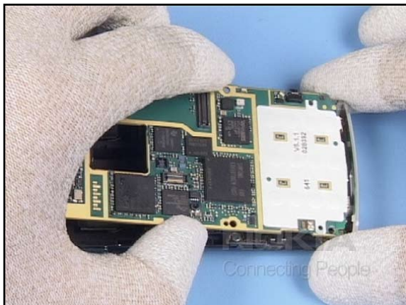
19. Insert the PWB into the CHASSIS, beginning from the bottom.
