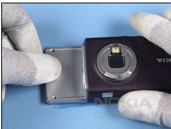
18. Slide the assembly into the second position to access the next treads.
