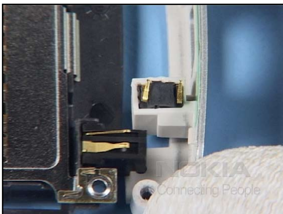
22. The BOTTOM COVER can be separated easily.
