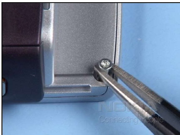
15. Insert two new screws.
