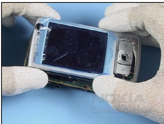
30. Bring the slider into position shown while placing it over the lower part.
