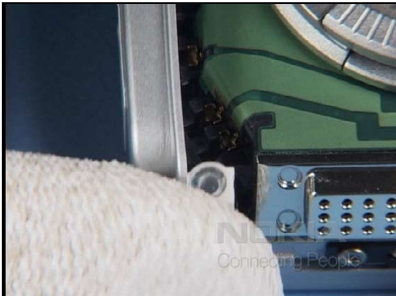
13. Lift up the TOP COVER ASSY first, then remove it.
