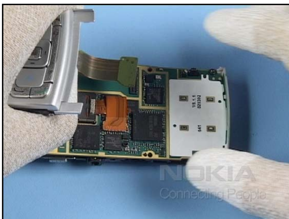
28. Position the upper block below the PWB.
