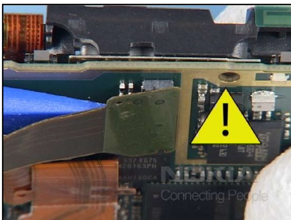
16. Be double careful while opening this connector. Do not destroy the hidden components underneath.
